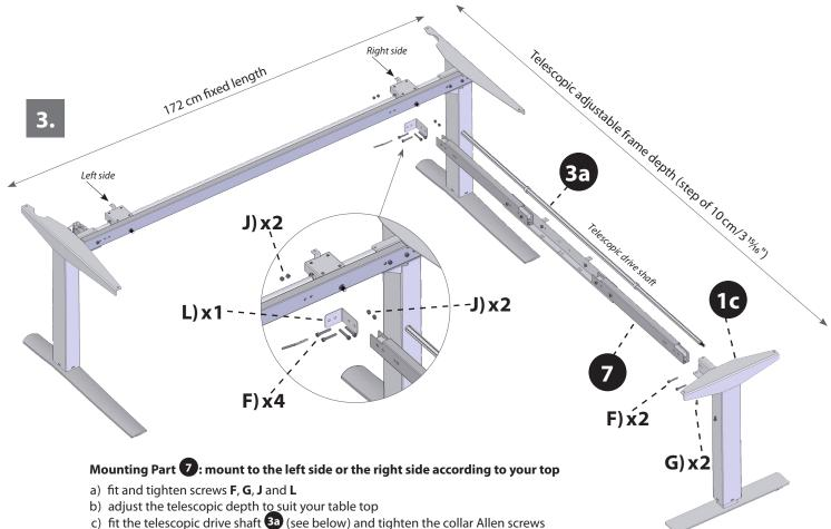
to lock the shaft length, making sure **X1** and **X2** are equal
